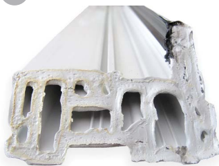
After Welding Corner Cut Open
